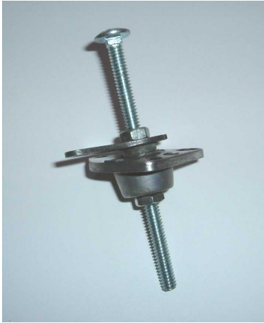
Fig 16. Substitute BC made from 1/4" bolt and 2 nuts
