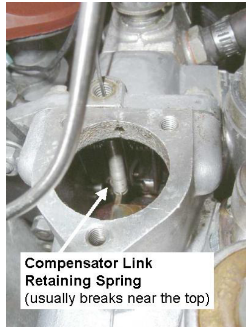
Fig 4. Compensator Link Retaining Spring.
