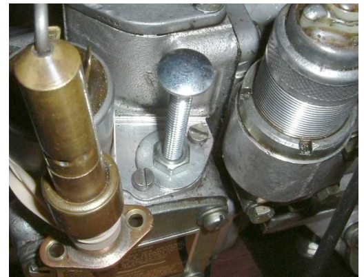
Fig 24. Emergency Substitute T/A installed. Note inoperative TA secured to prevent damage to TA pipe.
