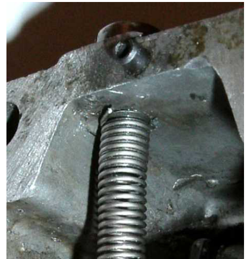
Fig 6. Retaining Spring upper attachment point
