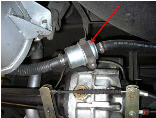
Fig 1. Rear Fuel Filter
