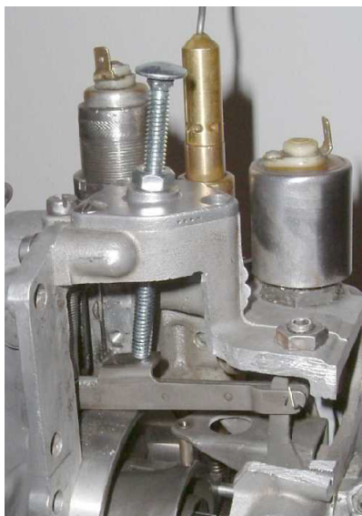
Fig 17. Dummy BC installed in cutaway of logic section. It is essentially a "fixed" BC now and will not adjust the pump mixture for changes in altitude and air density. Adjusting the length so as to engage the 7th notch of the vertical notched lever. (nominally 27 mm), will put it close enough for the engine to run.
