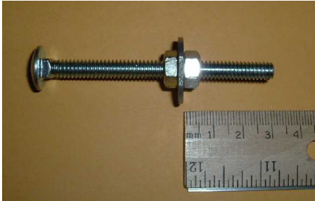
Fig 22. Emergency Substitute TA consisting of 1/4" x 3" stove bolt, two nuts, and washer. Nuts adjusted to give correct length.
