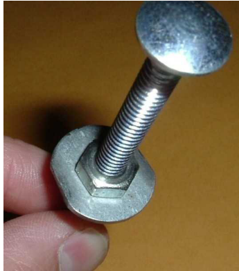
Fig 23. Emergency Substitute T/A Note filed off edges on washer in order to fit width of existing machine screws
