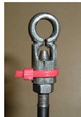
Fig 11. Cracked Rod End temporary repair with plastic wire tie.
