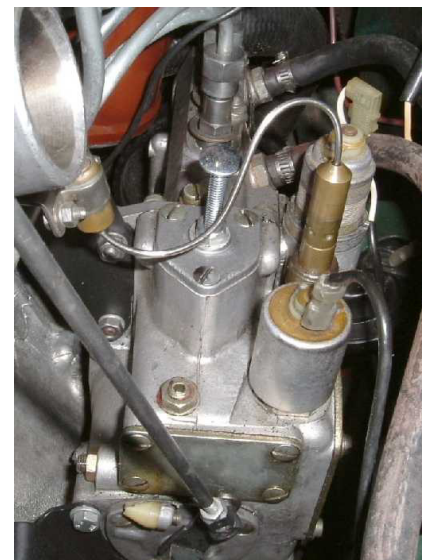
Fig 18. Dummy BC installed in car's injection pump.
