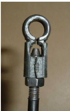
Fig 10. Cracked Rod End
