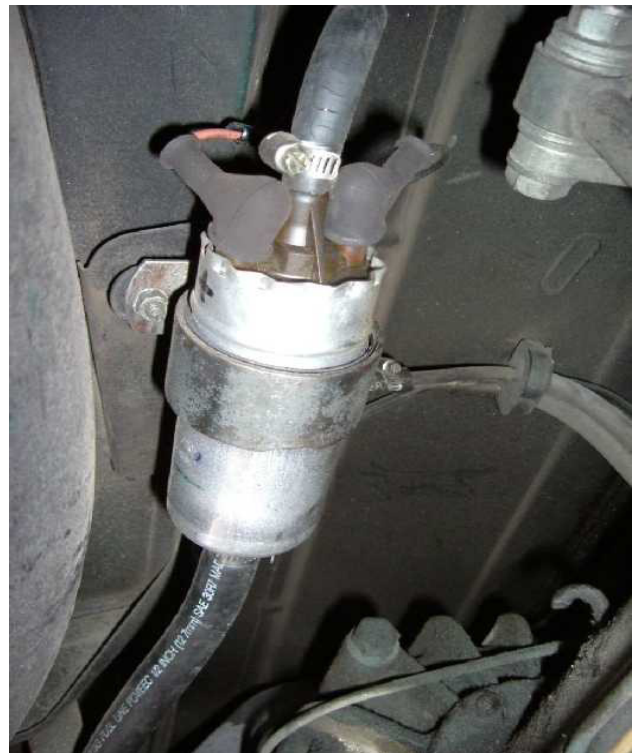
Fig 2. Fuel Supply Pump. Pictured pump is a Bosch L-Jet type. You may have the older model with 3 ports on one end, or two ports in an "L" shape, or even an original AEG pump.
