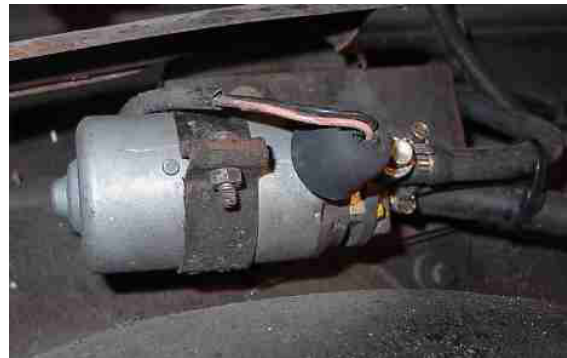
'69-'74 2-port Pump Installation (right axle area). Fig 1
