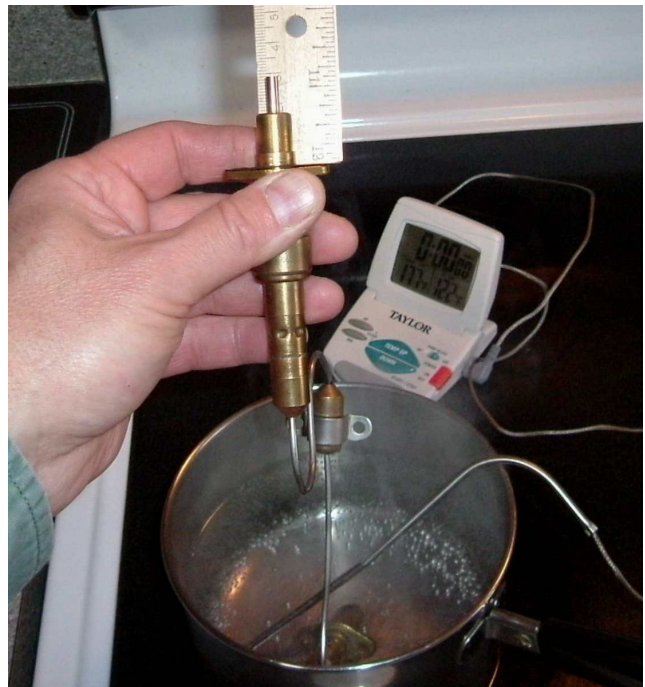
Fig 16. Testing the Thermostatic Actuator
