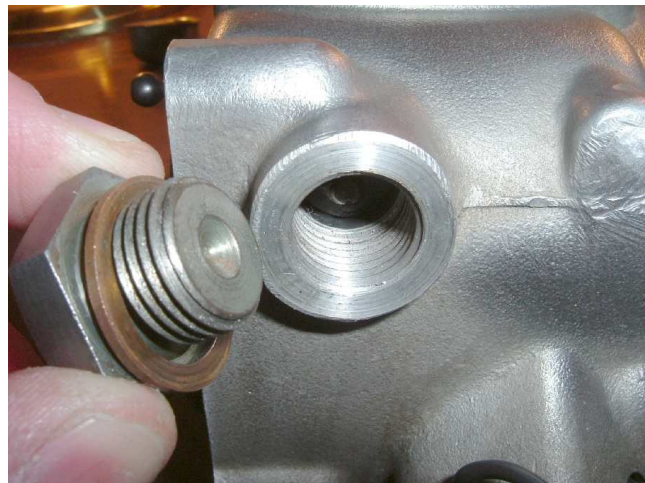
Fig 5. Cold Start Solenoid hydraulic piston bore
