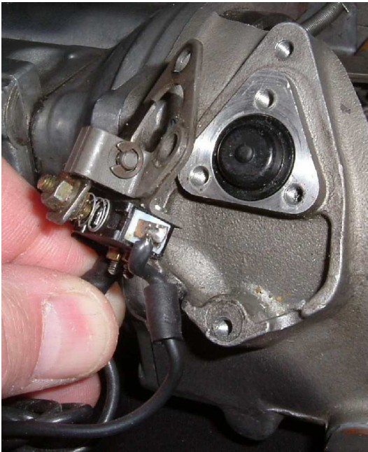
Fig 13. Removing microswitch assembly
