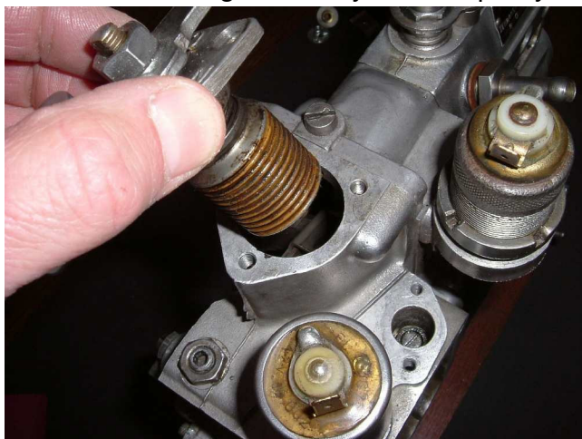
Fig 3. Removing the Barometric Compensator (BC).
