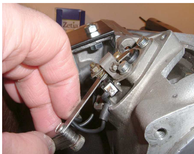
Fig 12. Checking the Microswitch adjustment
