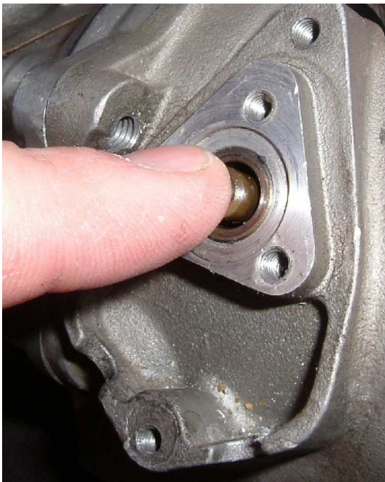
Fig 15. Testing spring in pushrod
