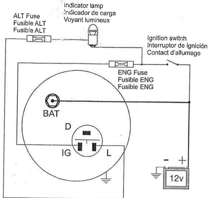
3. The BAT terminal must have battery voltage. This voltage is supplied directly from the battery and will be present whether the ignition switch is in the "ON" or "OFF" position. Failure to have voltage at this terminal will cause:
